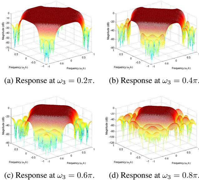
**Fig. 3.** Magnitude responses for the  $H_0(z)$  filter at  $\omega_3 = [0.2, 0.4, 0.6, 0.8]\pi$ .
