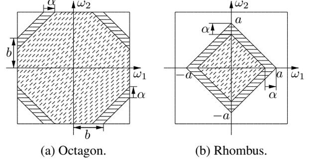
Fig. 2. Passband sections through the  $\omega_3$  axis.
