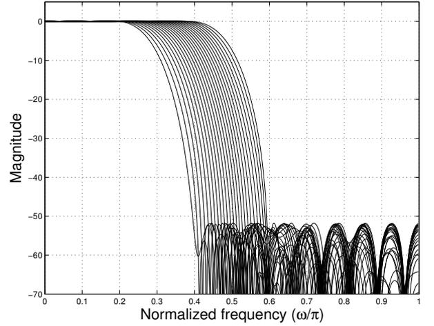
**Fig. 2.** Frequency responses of adjustable filters designed in Example 1 with  $K = 4$ , for 25 values of the parameter  $\theta \in [0.3\pi, 0.5\pi]$ .
