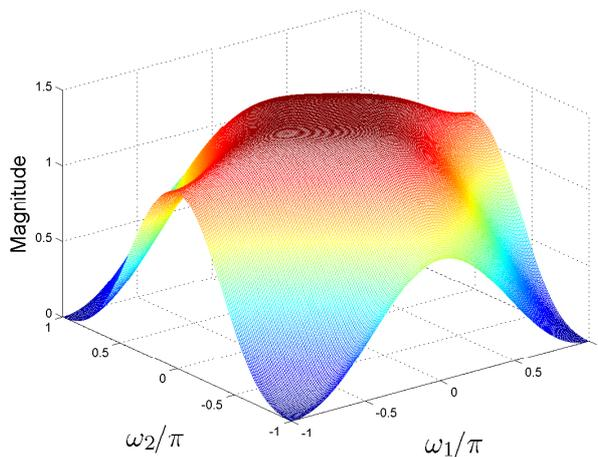
Fig. 4. Frequency response of filter designed in Example 2,  $\varepsilon = 10^{-6}$ .
