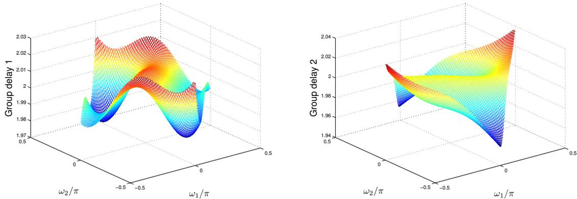
Fig. 3. Group delays in passband for the filter designed in Example 1,  $\varepsilon = 10^{-5}$ .
