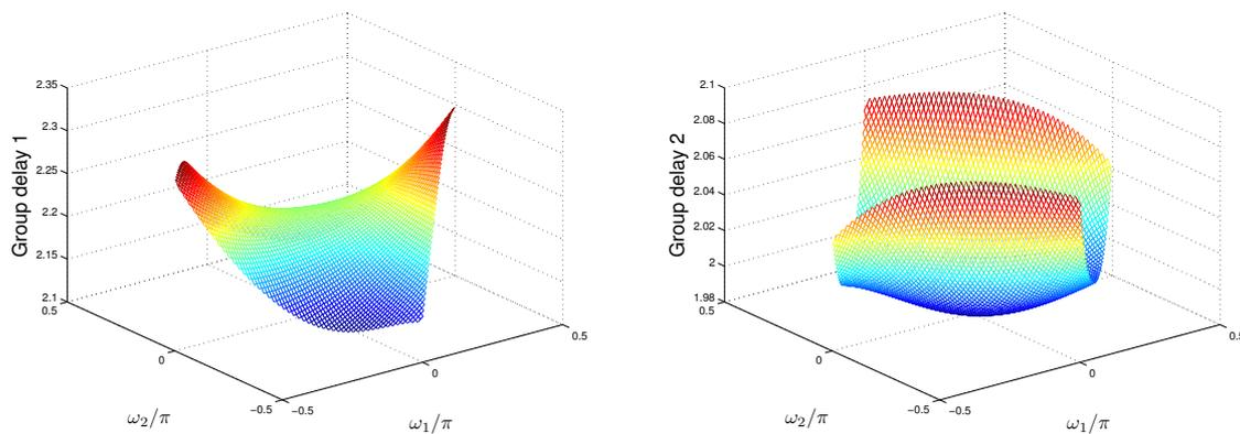
Fig. 5. Group delays in passband for the filter designed in Example 2,  $\varepsilon = 10^{-6}$ .
