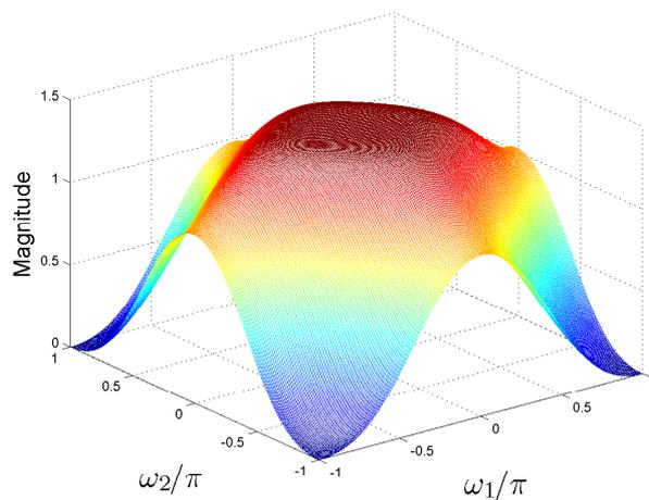
Fig. 2. Frequency response of filter designed in Example 1,  $\varepsilon = 10^{-5}$ .
