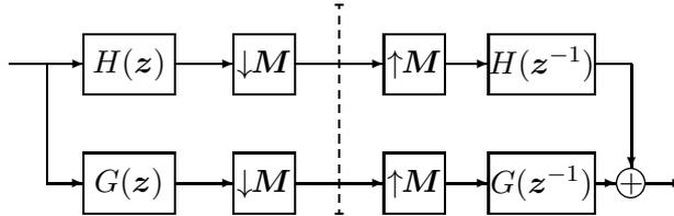
Fig. 1. 2-channel orthogonal filter bank.
