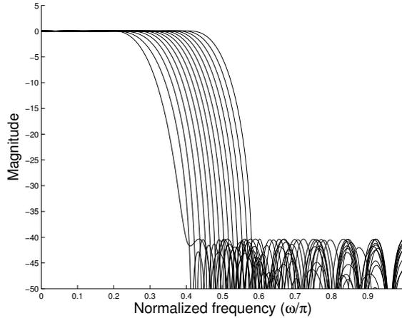
**Figure 1.** Frequency responses of a family of adjustable filters.
